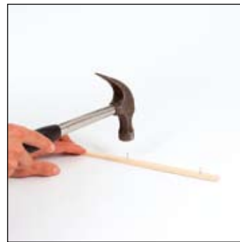
Take the piece that was snapped off earlier and mark the positions of the wires with a pen. Tap 3 nails in.
