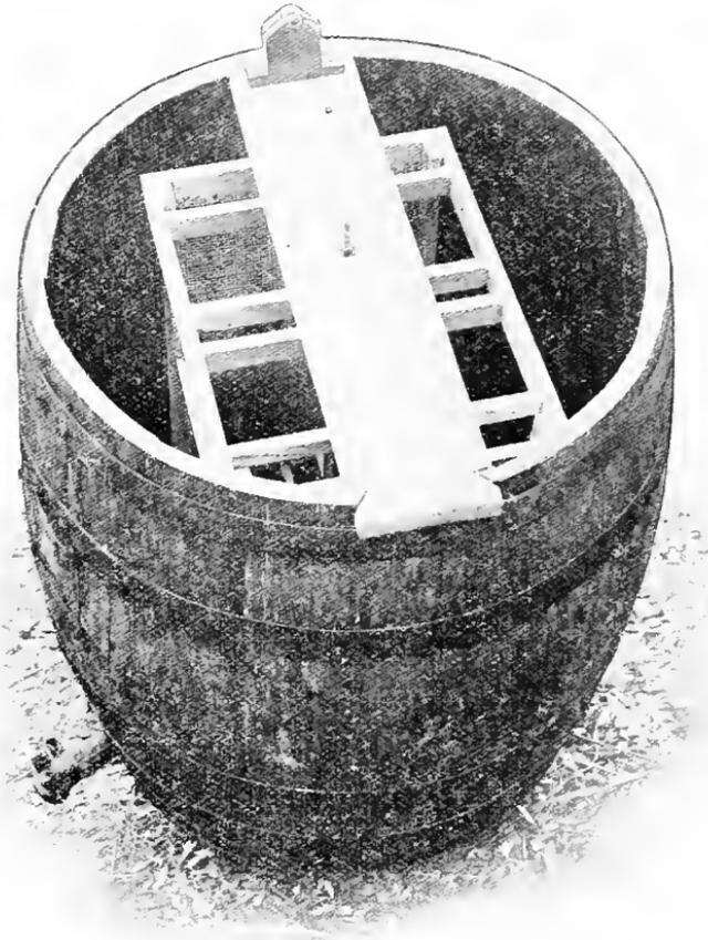
FIG. 3.—A home-made extractor. The frames filled with honey, after being uncapped with a knife, are placed in this machine and the honey thrown out by rapid turning with a crank. The honey is then drawn out by means of the spigot at bottom of the extractor. (Photo by Prof. Hutt).
